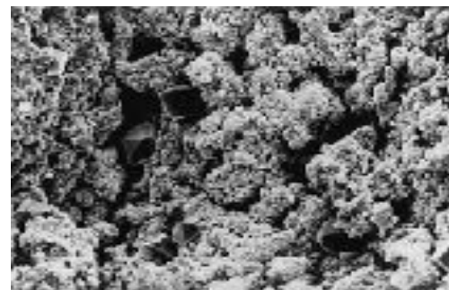
Battery Plate Desulfated by Reconditioner
