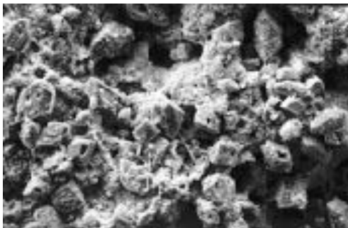
Battery Plate Partially Desulfated by Reconditioner
