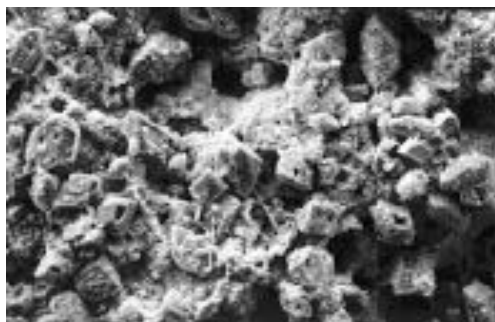
Battery Plate Partially Desulfated by Reconditioner
