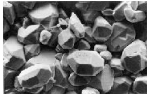
Sulfated Battery Plate
