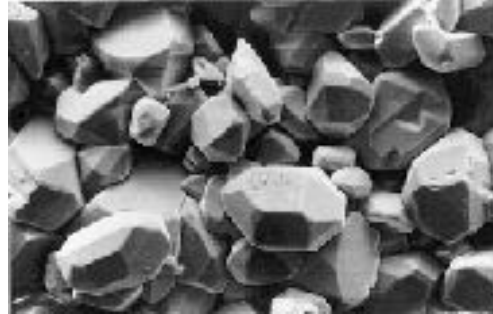
Sulfated Battery Plate
